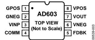
Figure 3. 8-Lead CERDIP Pin Configuration
