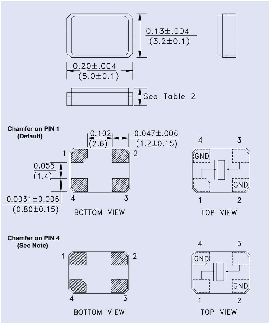
**Note:** Due to the availability of raw materials, this part may be manufactured with the chamfer on pin 4. Be advised that this does not affect the electrical characteristics of the crystal in any way.
