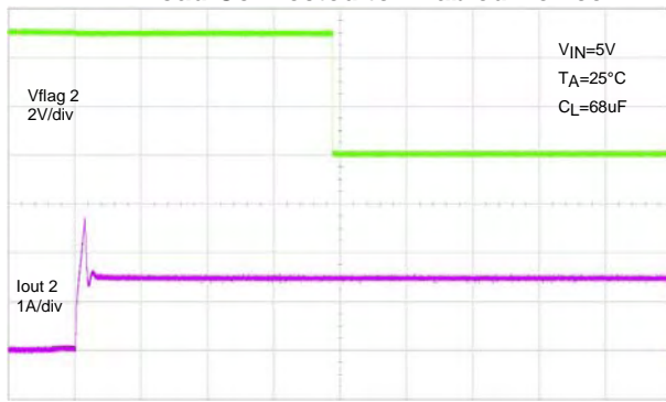
1 Ω Load Connected to Enabled Device
