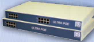
Rack Mountable Midspans
