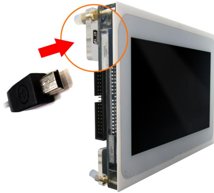
Figure 1-3 External USB Power Connection Setup
