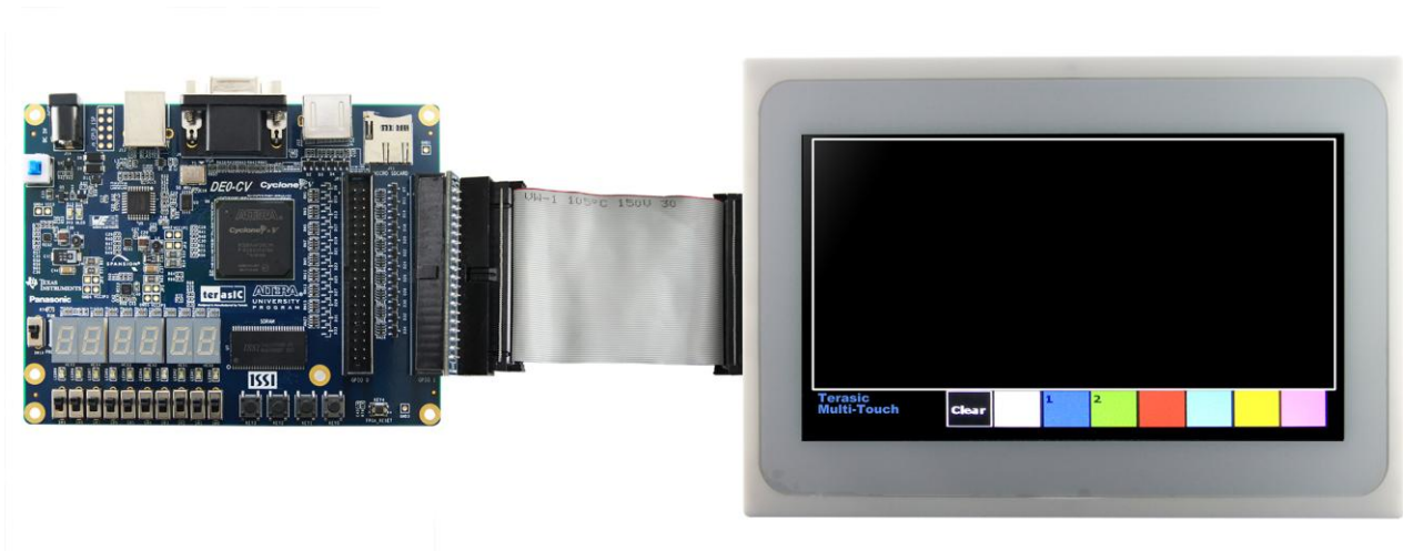
Figure 5-7 Hardware Setup with DE0-CV
