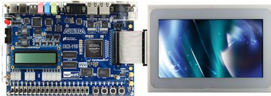
Figure 5-4 Hardware Setup with DE2-115
