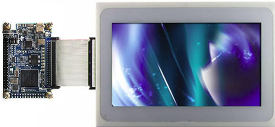
Figure 5-6 Hardware Setup with DE0-Nano
