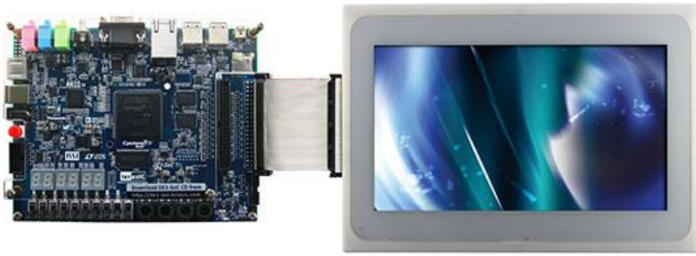
Figure 5-5 Hardware Setup with DE1-SoC
