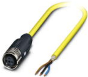
Sensor/Actuator cable, 3-position, PVC, Yellow RAL 1021, shielded, Free cable end, on Socket straight M12-SPEEDCON, A-coded, Cable length: 2 m
