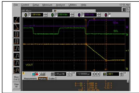
FIGURE 2-99: Half-Scale Settling Time (C00h to 400h) (MCP4726).
