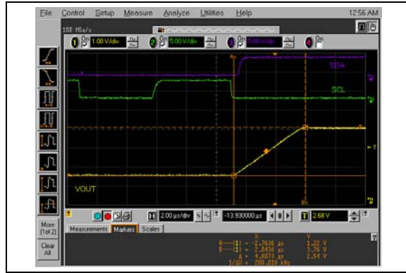
FIGURE 2-98: Half-Scale Settling Time (400h to C00h) (MCP4726).
