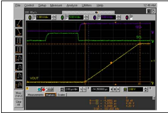
FIGURE 2-96: Full-Scale Settling Time (000h to FFFh) (MCP4726).
