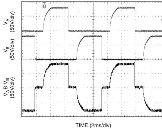
Figure 6. Typical EL Driver for 2in<sup>2</sup> Lamp with C<sub>S</sub> = 0.1µF
