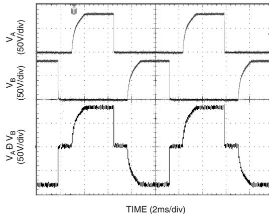
Figure 5. Typical 100Hz EL Driver for 3in<sup>2</sup> Lamp
