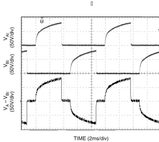
Figure 7. Typical EL Driver for 2in<sup>2</sup> Lamp with 560µH inductor
