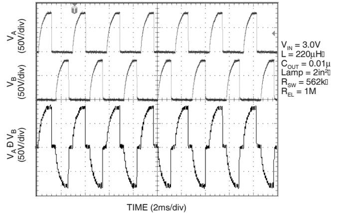
**Figure 4. 360Hz Output Waveform**
