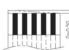
Tolerance of Cutting Tilt
