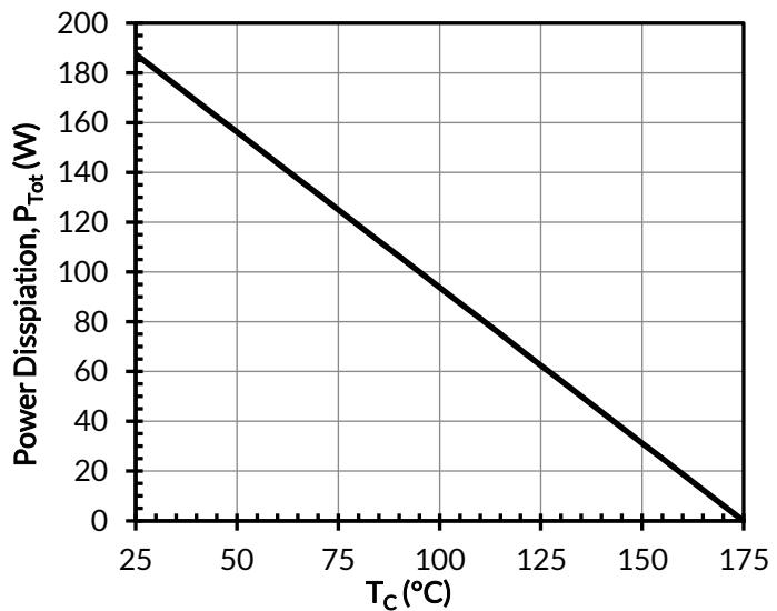
Figure 4. Power dissipation
