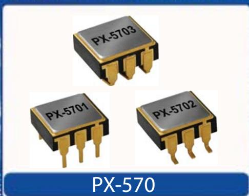
Vectron offers a High Temperature Crystal Oscillator (PX-570) product platform for extreme environment applications. In addition to its wide operating temperature range, PX-570 HTXO is also ideal for high shock & vibration applications. PX-570's unique package design offers small ceramic package footprint, as well as providing both through-hole mounting and surface mount options.
