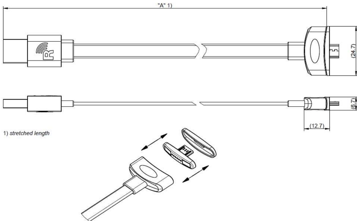
All dimensions are in mm; tolerances according to ISO 2768 c
