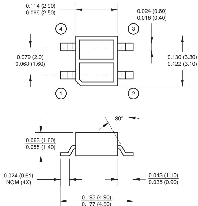
PIN 1 ANODE      PIN 3 COLLECTOR
