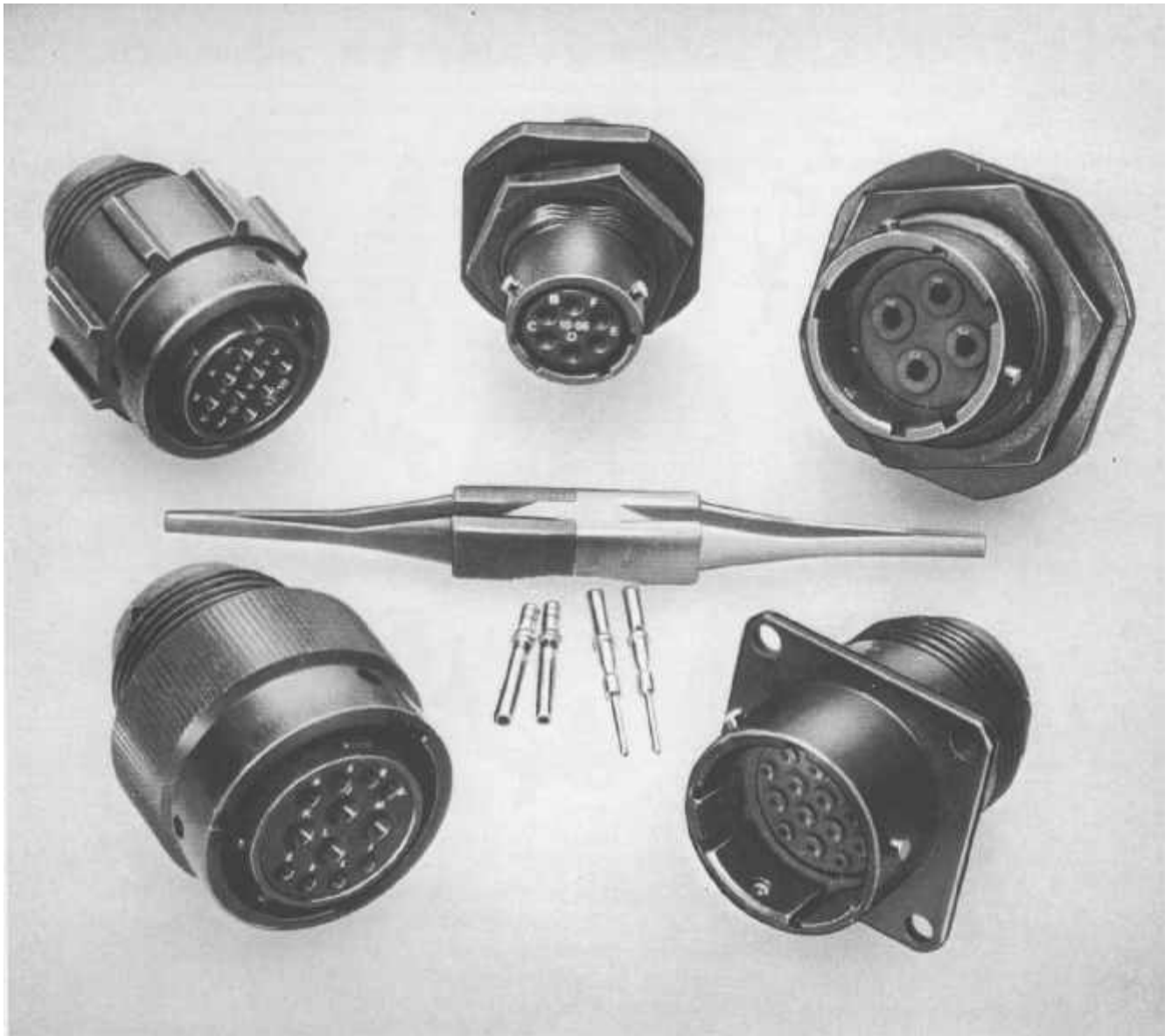
High temperature Miniature Bayonet Lock Connectors with rear insertable, rear release crimp contacts. Connectors to EL 2112 Patt. 602 DEF STAN 59-56 & PAN 6432 -1 & -4.
