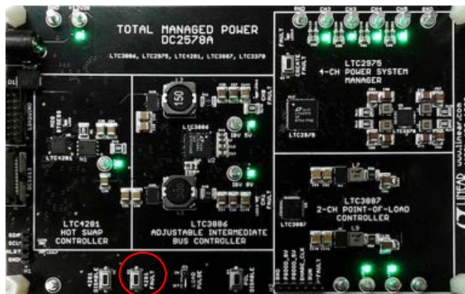
Figure 9. LTC4281 Fault Button
