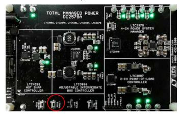
Figure 9. LTC4281 Fault Button
