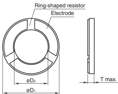
**PLANE SURFACE ELECTRODE TYPE(5-ELECTRODE)**
