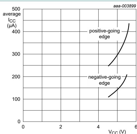
Fig. 13. Average additional supply current as a function of  $V_{CC}$  for 74HCT132;
