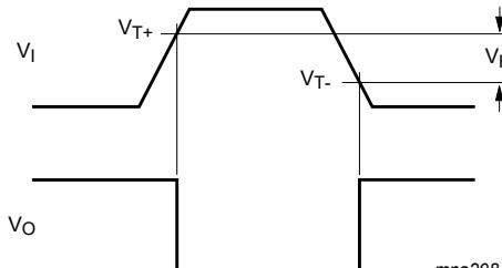
Fig. 9. Transfer characteristics definitions
