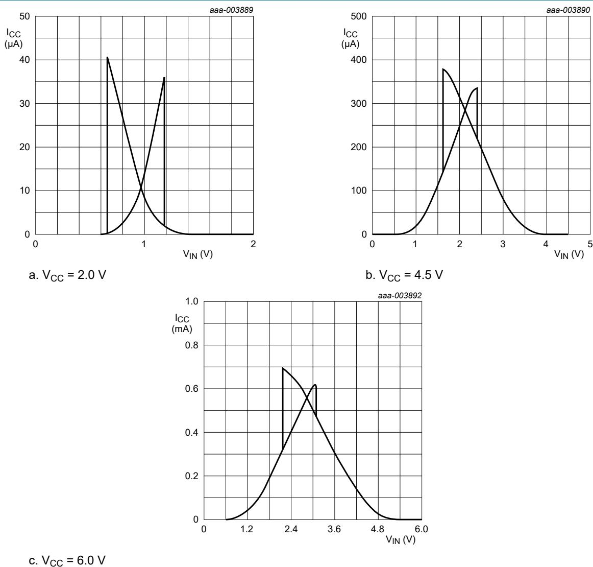
**Fig. 10. Typical 74HC132 transfer characteristics**
