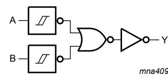
Fig. 3. Logic diagram (one Schmitt trigger)
