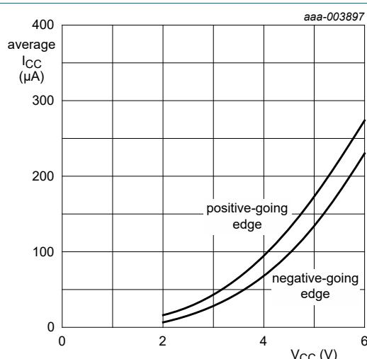
Fig. 12. Average additional supply current as a function of  $V_{CC}$  for 74HC132;
