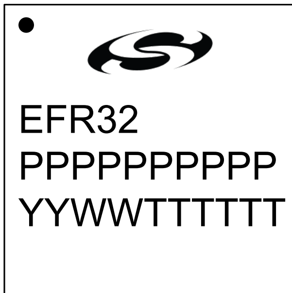
Figure 8.3. RQFN32 Package Marking
