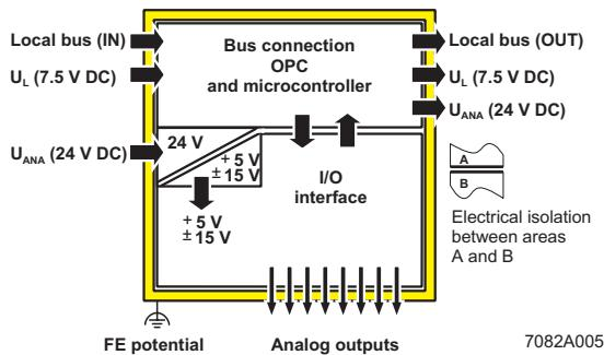
Figure 3 Electrical isolation of the individual function areas
