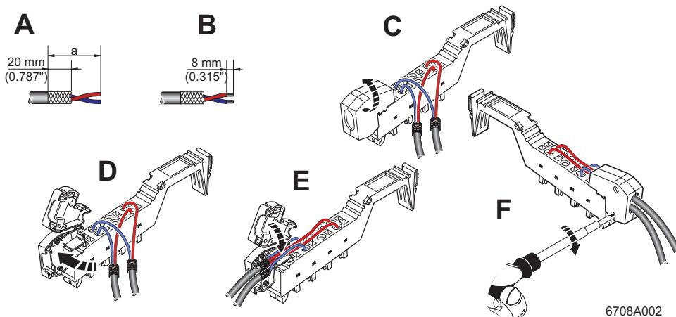
Figure 7 Connecting the shield using the shield connector
