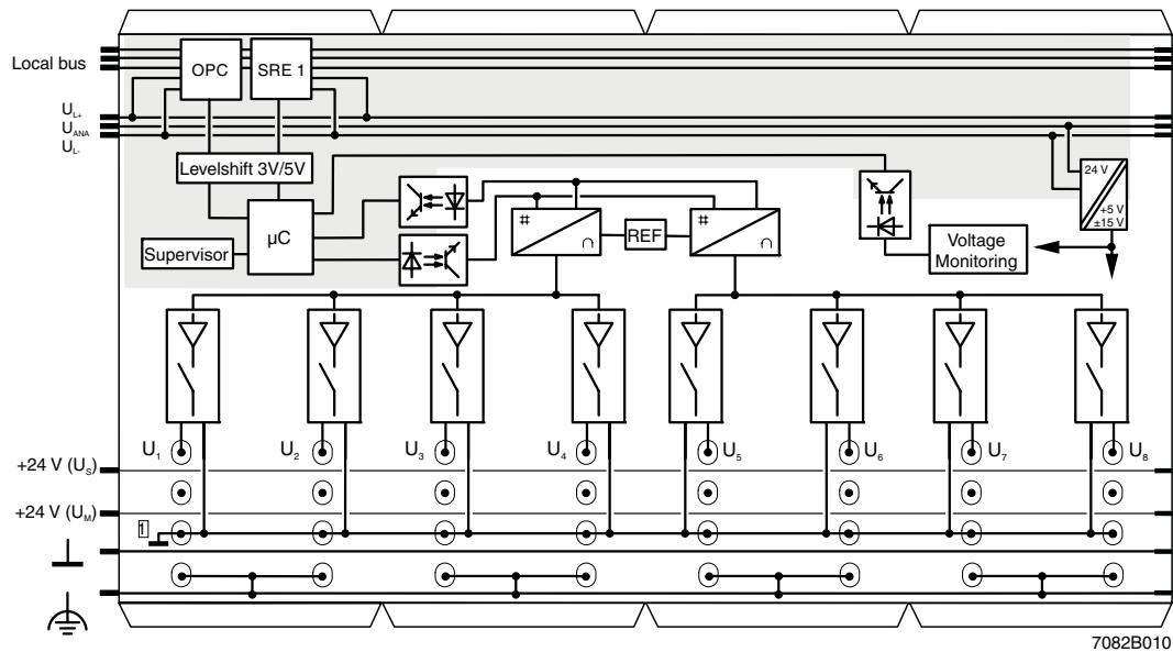
Figure 2 Internal wiring of the terminal points
