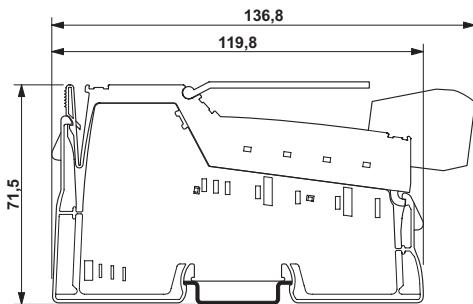
Housing dimensions (width x height x depth)
