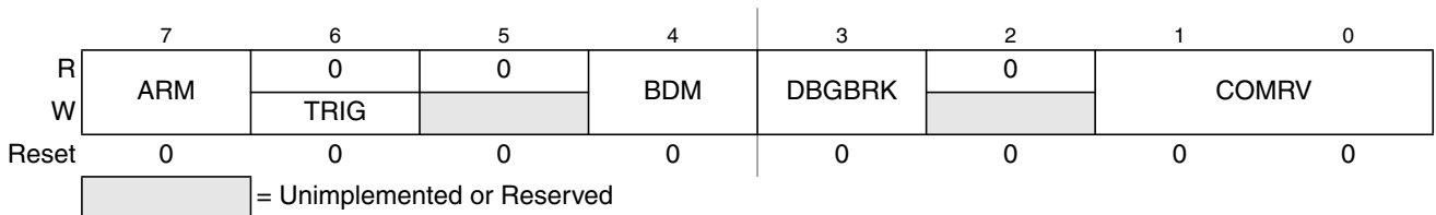
Figure 6-3. Debug Control Register (DBGC1)
