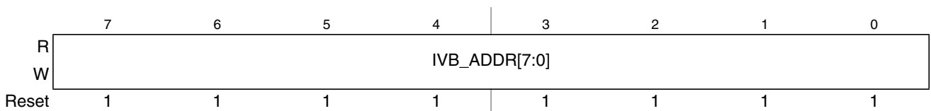
Figure 7-2. Interrupt Vector Base Register (IVBR)
