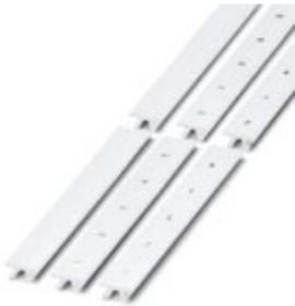
Zack marker strip, Can be ordered: Strip, white, Labeled according to customer specifications, Mounting type: Snap into tall marker groove, For terminal block width: 15.2 mm, Lettering field: 10.5 x 15.1 mm
