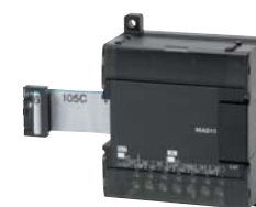
■ Analog I/O Unit CP1W-MAD11 ● Analog inputs: 2 (resolution: 6,000) ● Analog outputs: 1 (resolution: 6,000)
