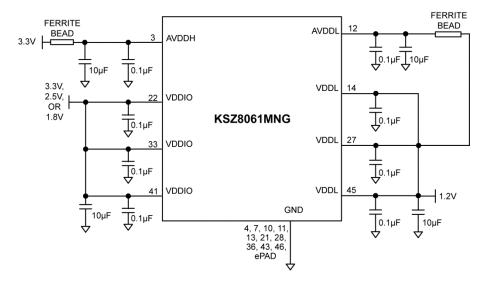
Figure 13. KSZ8061MNG Power and Ground Connections
