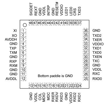
Figure 2. 48-Pin 7mm x 7mm QFN
