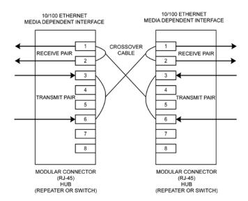
Figure 8. Typical Crossover Cable Connection
