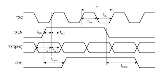
Figure 14. MII Transmit Timing (10Base-T)
