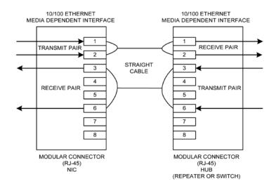
Figure 7. Typical Straight Cable Connection
