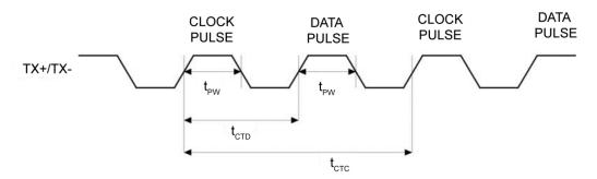
Figure 18. Auto-Negotiation Fast Link Pulse (FLP) Timing
