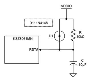
Figure 21. Recommended Reset Circuit
