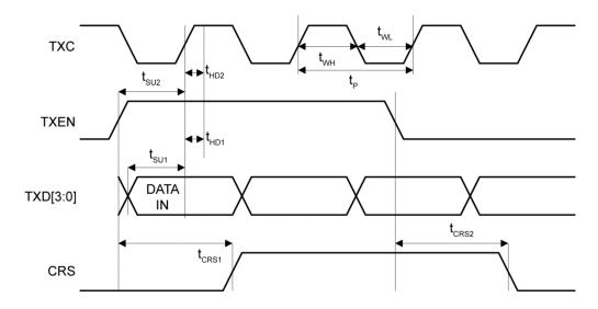
Figure 16. MII Transmit Timing (100Base-TX)
