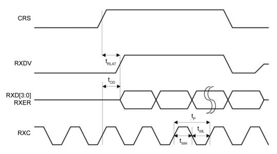
Figure 15. MII Receive Timing (10Base-T)
