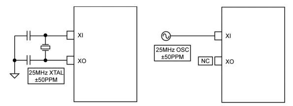
Figure 23. 25MHz Crystal/Oscillator Reference Clock Connection
