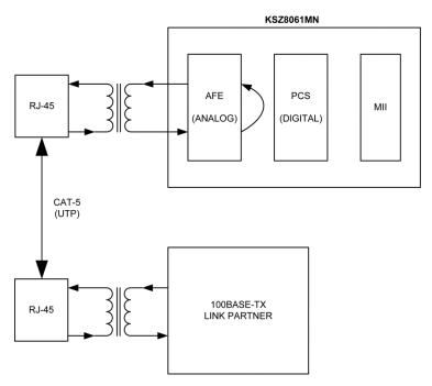
Figure 10. Remote (Analog) Loopback
