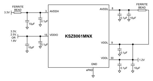
Figure 12. KSZ8061MNX Power and Ground Connections
