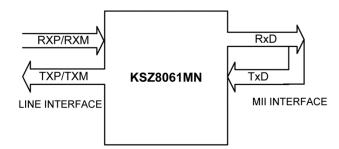
Figure 6. KSZ8061MN Back-to-Back for MII Bus Loopback
