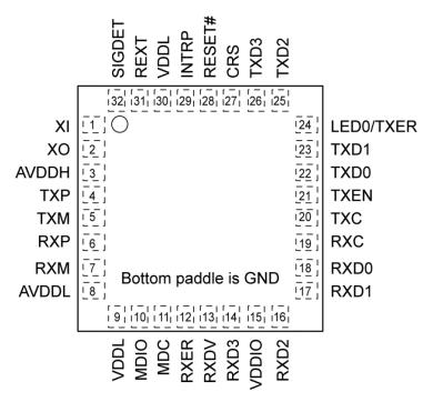
Figure 1. 32-Pin 5mm x 5mm QFN or WQFN
