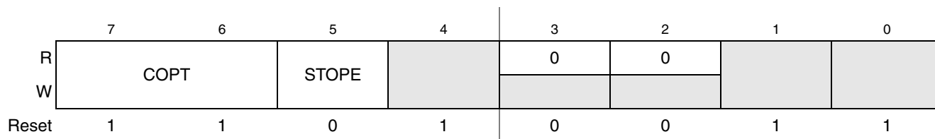
Figure 5-5. System Options Register (SOPT1)
