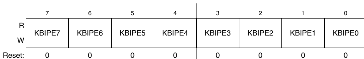
Figure 8-4. KBI Pin Enable Register
