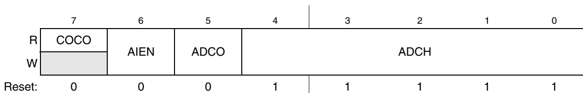
Figure 10-3. Status and Control Register (ADCSC1)
