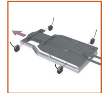
Measuring Car Body Widths (ZS-HLDS10)
