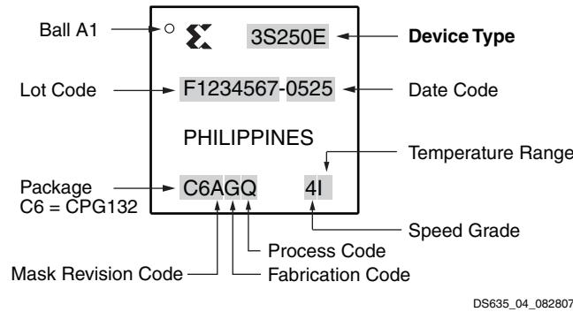
*Figure 4: XA Spartan-3E FPGA CPG132 Package Marking Example*
