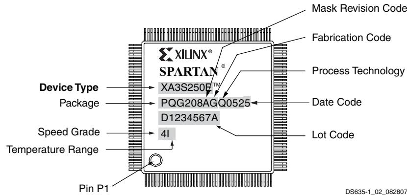
*Figure 2: XA Spartan-3E FPGA QFP Package Marking Example*
