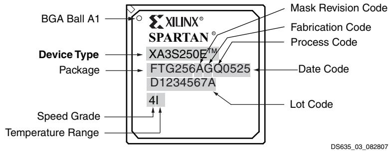
*Figure 3: XA Spartan-3E FPGA BGA Package Marking Example*
