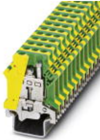
Ground terminal block with screw connection, cross section: 0.5 - 10 mm 2 , AWG: 20 - 6, width: 10.2 mm, color: green-yellow
