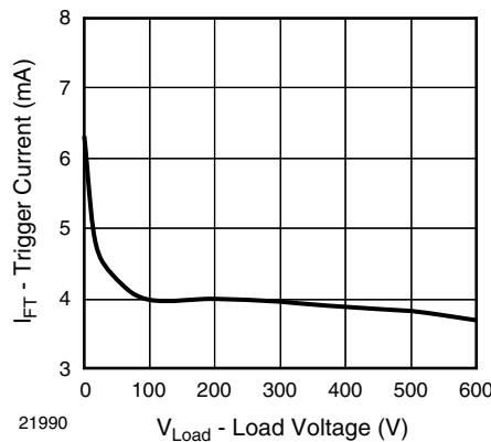
Fig. 11 - Trigger Current vs. Load Voltage
