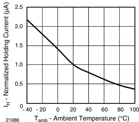
Fig. 8 - Normalized Holding Current vs. Ambient Temperature
