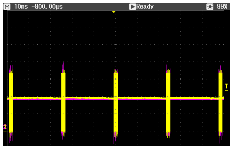
Figure 4-5. Debug Lines Floating Between Debug Data Sends (30 Bytes, ~2 ms to Send)
