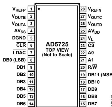
Figure 6. Pin Configuration Diagram
