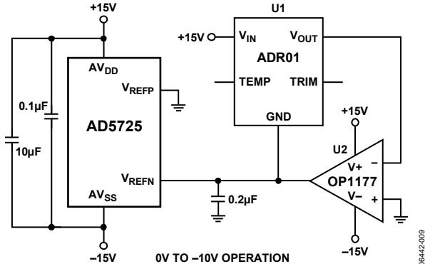
Figure 29. Unipolar  $-10\text{ V}$  Operation
