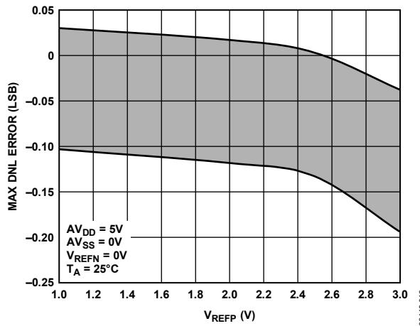
Figure 8. DNL vs.  $V_{REFP}$  ( $V_{SUPPLY} = +5 V$ )
