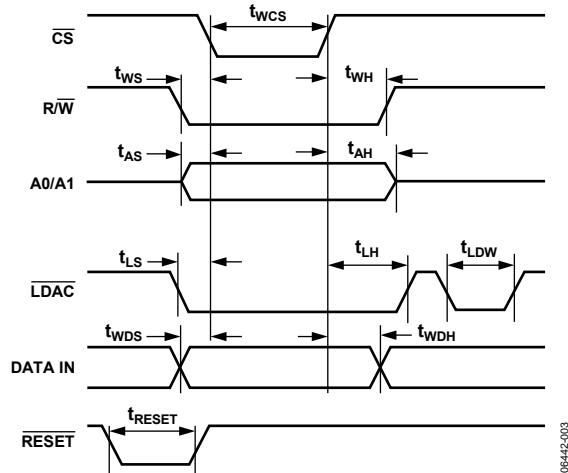
Figure 3. Data Write Timing
