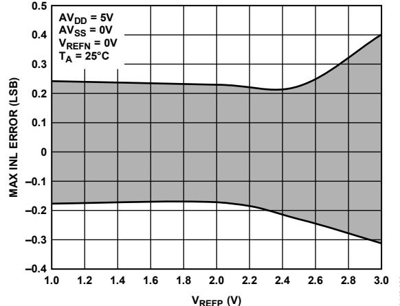
Figure 10. INL vs.  $V_{REFP}$  ( $V_{SUPPLY} = +5 V$ )
