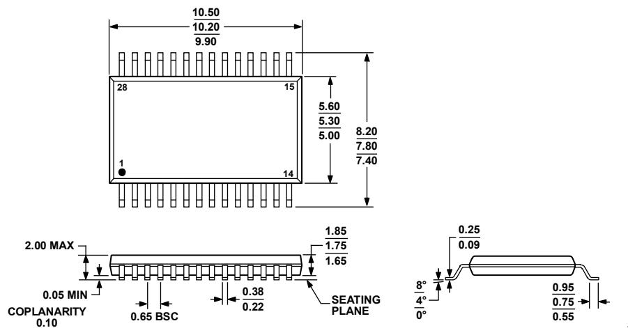
Figure 31. 28-Lead Shrink Small Outline Package [SSOP]
