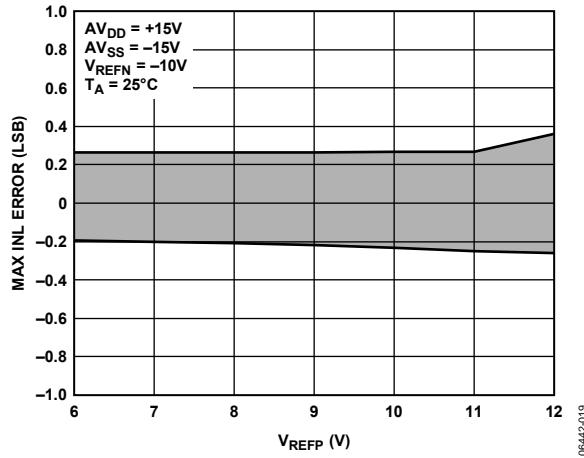
Figure 9. INL vs.  $V_{REFP}$  ( $V_{SUPPLY} = \pm 15 V$ )
