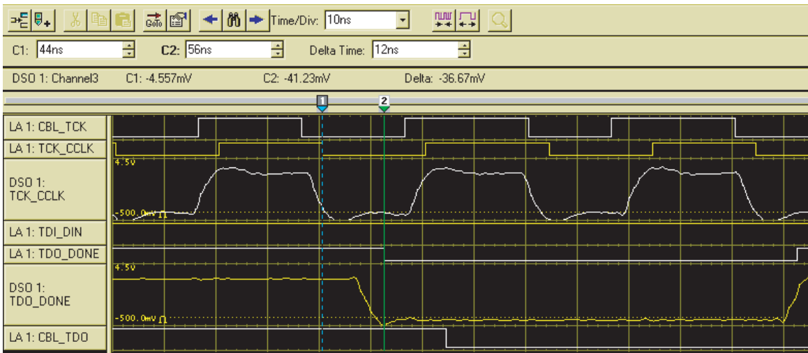
Figure 20: TDO_DONE_MISO Timing with Respect to TCK_CCLK_SCK (TCK_CCLK_SCK to TDO_DONE_MISO Delay)
