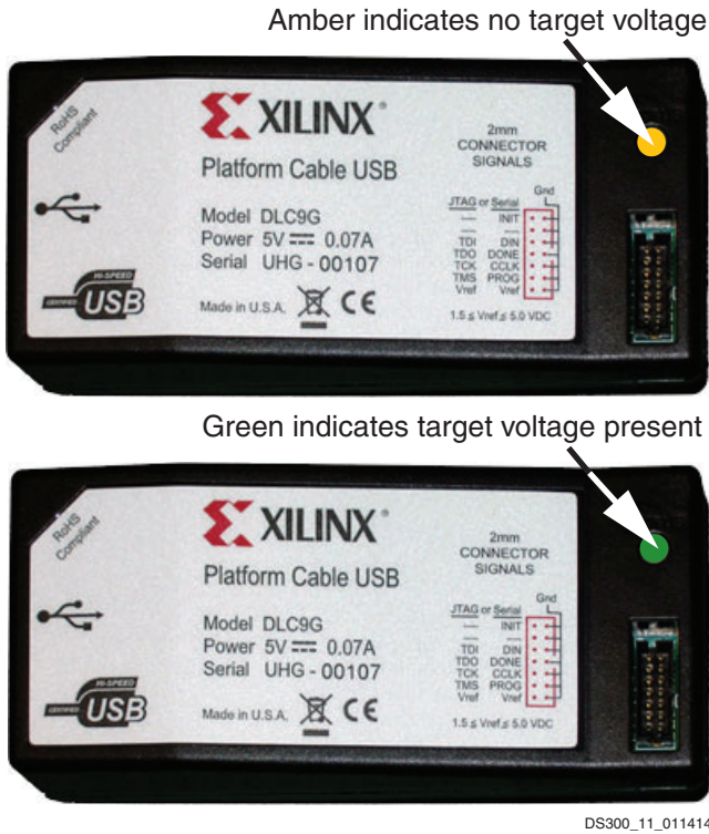
Figure 11: Status LEDs Indicating Target Voltage
