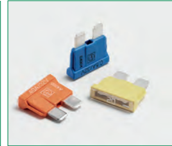
FKS AT0® 32V Fast-Acting Automotive Copper Blade Fuse Amps (A): 1-4, 5, 7.5, 10, 15, 20, 25, 30, 35, 40
