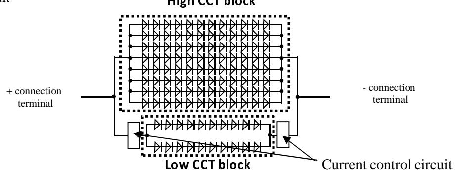
High CCT block 12 series × 8 parallel = 96 pcs of LEDs
