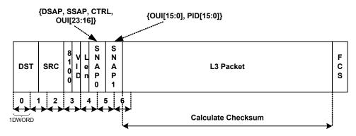
Figure 3.6 Ethernet Frame with VLAN Tag and SNAP Header
