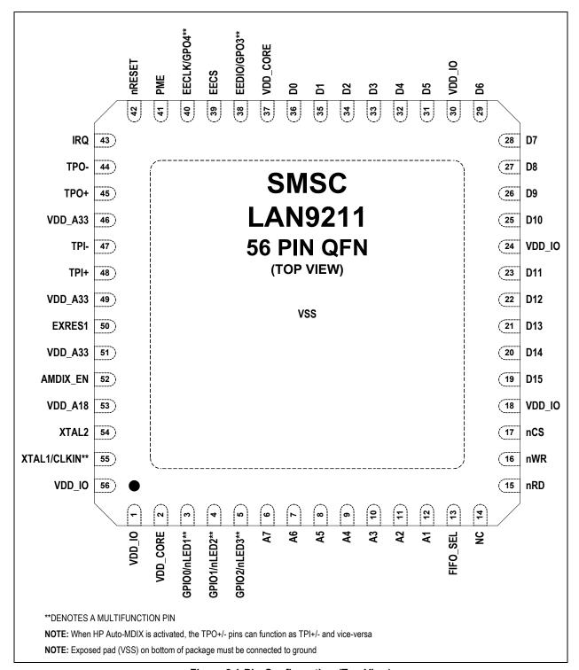
Figure 2.1 Pin Configuration (Top View)
