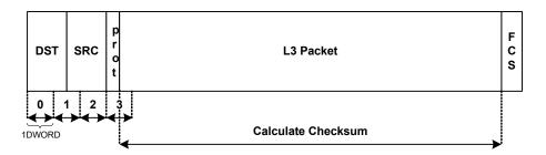
Figure 3.3 Type II Ethernet Frame
