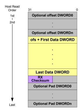
Figure 3.27 RX Packet Format with RX Checksum
