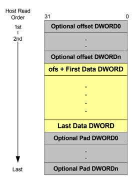
Figure 3.26 RX Packet Format
