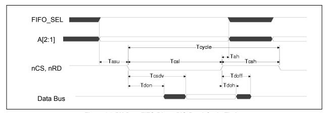
Figure 6.3 RX Data FIFO Direct PIO Read Cycle Timing
