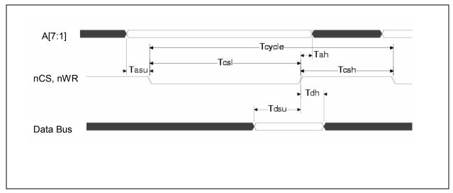
Figure 6.5 PIO Write Cycle Timing
