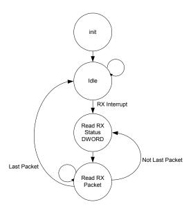
Figure 3.24 Host Receive Routine Using Interrupts
