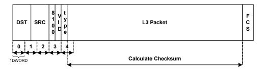
Figure 3.4 Ethernet Frame with VLAN Tag
