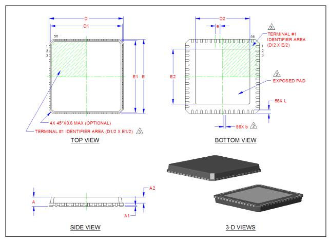
Figure 8.1 56 Pin QFN Package Definition
