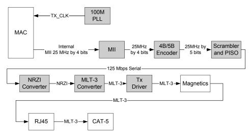
Figure 4.1 100Base-TX Data Path
