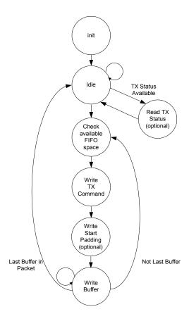
Figure 3.19 Simplified Host TX Flow Diagram
