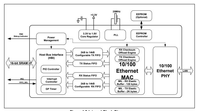
Figure 1.2 Internal Block Diagram
