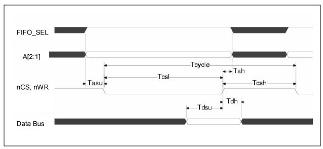
Figure 6.6 TX Data FIFO Direct PIO Write Timing
