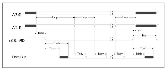
Figure 6.2 PIO Burst Read Cycle Timing
