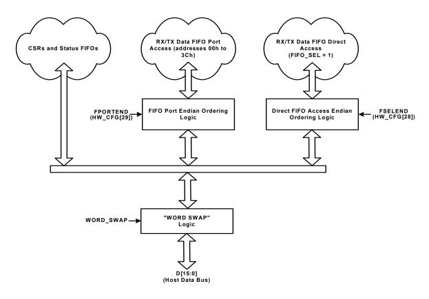
Figure 3.8 LAN9211 Host Data Path Diagram
