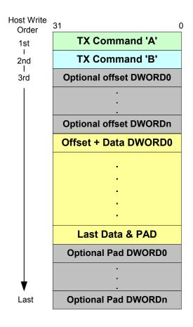
Figure 3.20 TX Buffer Format
