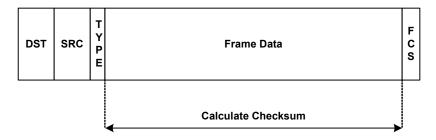
Figure 3.2 RXCOE Checksum Calculation
