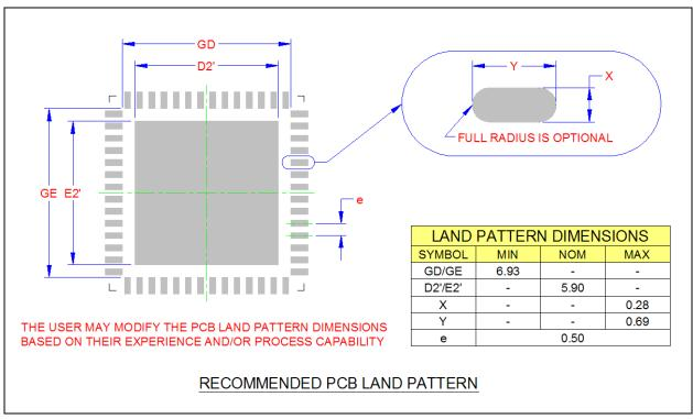
Figure 8.2 56 Pin QFN Recommended PCB Land Pattern
