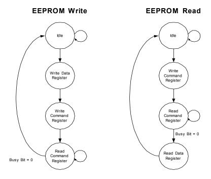
Figure 3.10 EEPROM Access Flow Diagram
