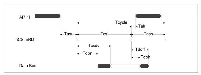
Figure 6.1 PIO Read Cycle Timing
