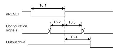
Figure 6.7 Reset Timing
