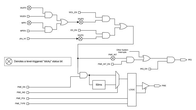
Figure 3.18 PME and PME\_INT Signal Generation
