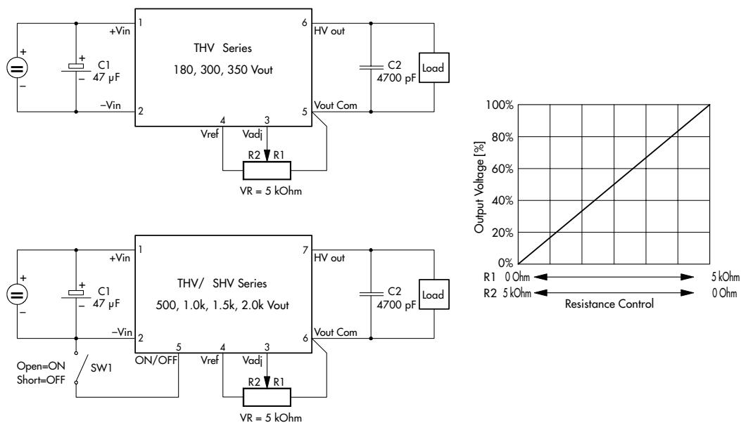
Connection for remote control voltage control
