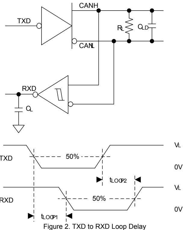
Figure 2. TXD to RXD Loop Delay
