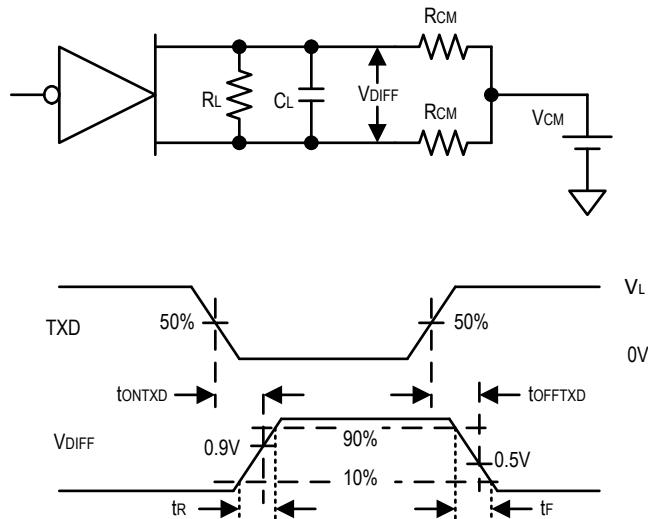
Figure 1. - Transmitter Test Circuit and Timing Diagram
