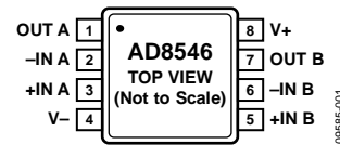
Figure 1. AD8546 (8-Lead MSOP)
