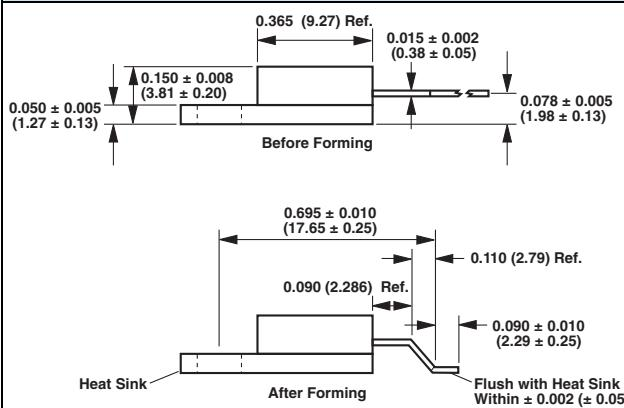
**FIGURE 6 - VPR221SZ DIMENSIONS** in inches (millimeters)
