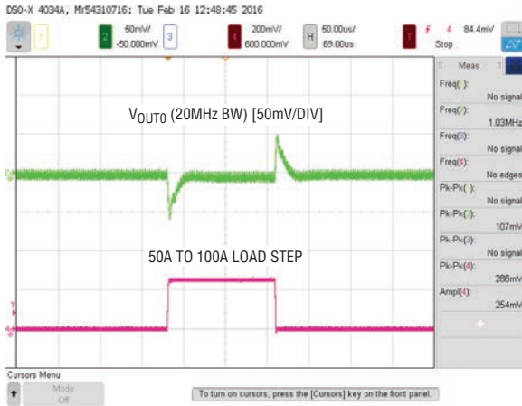
Figure 6. Output Voltage V_{OUTO} vs Load Current ( V_{OUTO} RANGE = 1)
