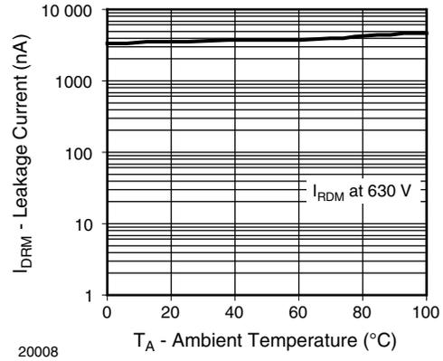
Fig. 4 - Leakage Current vs. Ambient Temperature
