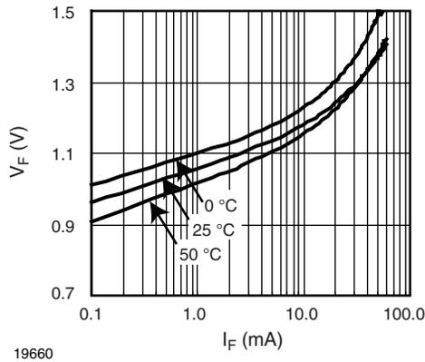
Fig. 2 - Diode Forward Voltage vs. Forward Current
