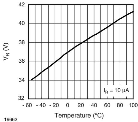
Fig. 3 - Diode Reverse Voltage vs. Temperature
