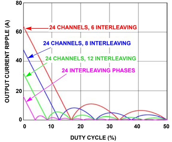
FIGURE 17. OUTPUT CURRENT RIPPLE vs DUTY CYCLE, PHASE COUNT
