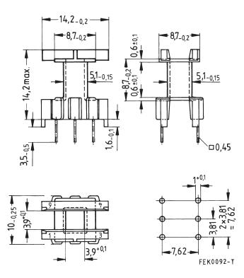
Hole arrangement View in mounting direction
