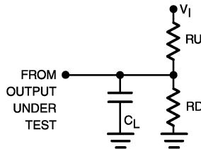
Note: Input driven by  $50\Omega$  source terminated in  $50\Omega$
