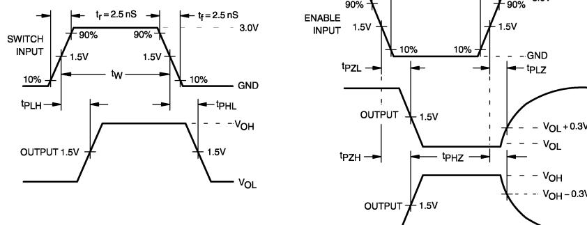
FIGURE 2. AC Waveforms
