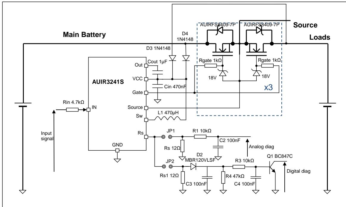
On the Demoboard, D4 is shorted and D3 is not connected.
