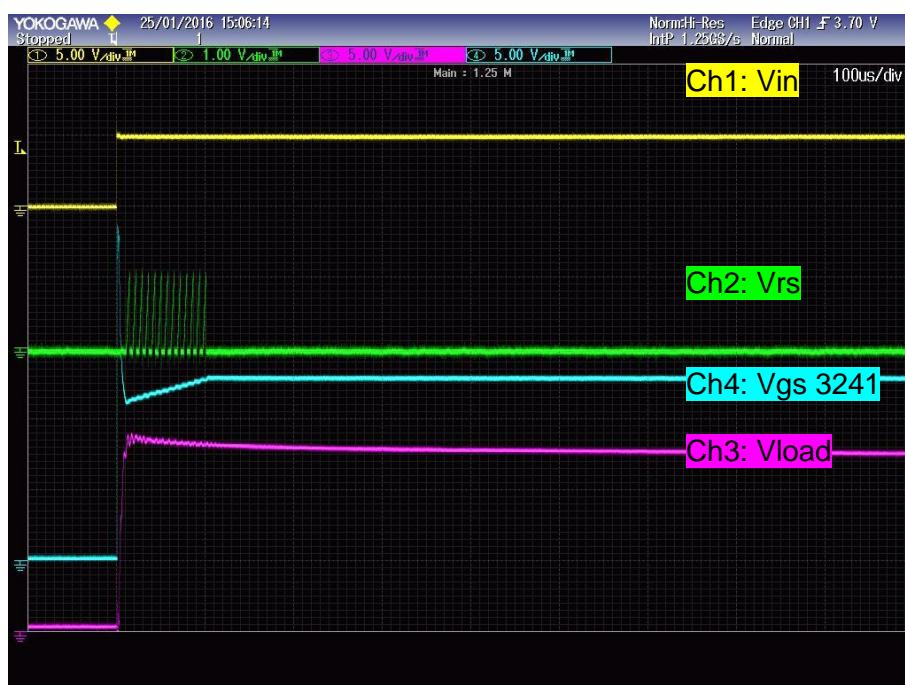
**Turn on with a Gate-Source resistor: R<sub>gs</sub>= 100Ω**
