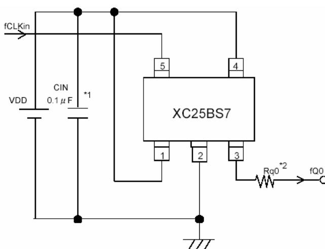
\*1:  $C_{IN}$  (by-pass capacitor, 0.1 µF) should be connected to the IC as close as possible.
