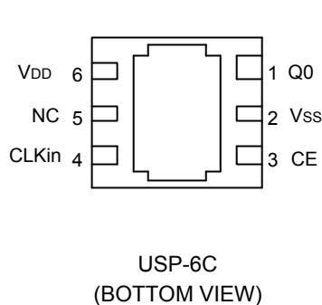
\* The dissipation pad (TAB) of the bottom view of the USP-6C package should be connected to the V<sub>SS</sub> (No. 2) pin.
