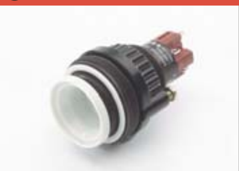
Illuminated pushbutton actuator for raised and flush mount, black plastic, solder terminal, snap-action, gold over silver contacts
