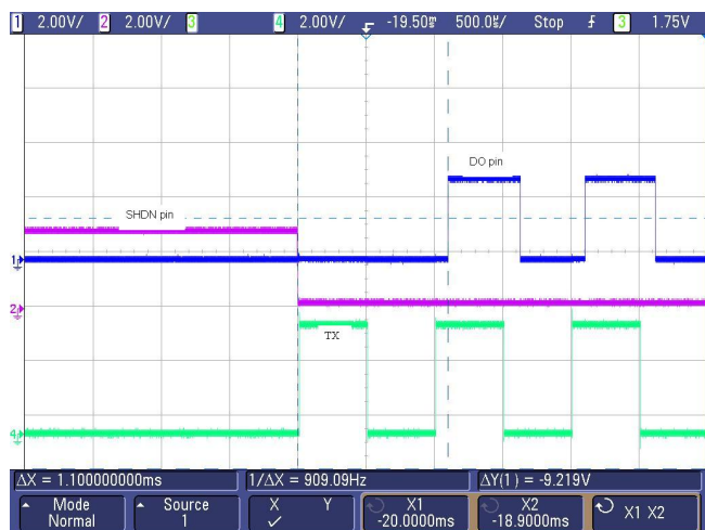
Figure 13. Time-to-Preamble Data after Shut Down Cycle, Room Temperature
