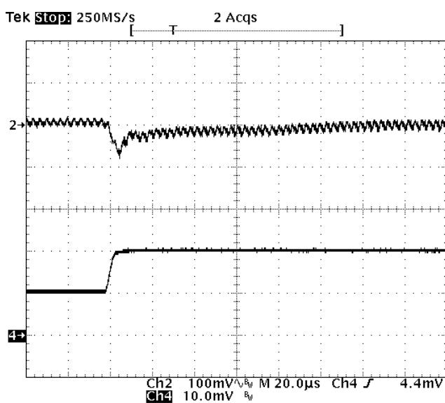
**Fig-2.0V-6:** Output voltage response for  $V_{out}=2.0V$  to positive load current step change from 5A to 10A with slew rate of  $5A/\mu s$  at  $V_{in}=12V$ .  $C_o=47\mu Fx2$  ceramic.
