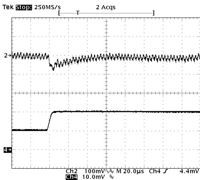
**Fig-5.0V-6:** Output voltage response for  $V_{out}=5.0V$  to positive load current step change from 5A to 10A with slew rate of  $5A/\mu s$  at  $V_{in}=12V$ .  $C_o=47\mu Fx2$  ceramic.
