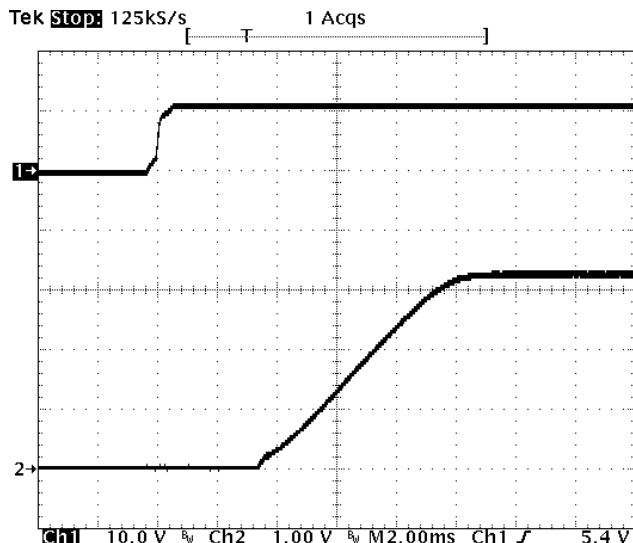
**Fig-3.3V-4:** Turn-on transient for  $V_{out}=3.3V$  with application of  $V_{in}$  at full rated load current (resistive) and  $47\mu Fx2$  external capacitance at  $V_{in}=12V$ .
