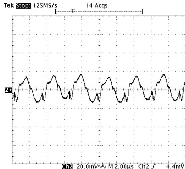
**Fig-5.0V-5:** Output voltage ripple (20mV/div.) for  $V_{out}=5.0V$  at full rated load current into a resistive load with external capacitance  $47\mu Fx2$  ceramic +  $1\mu F$  ceramic at  $V_{in}=12V$ .
