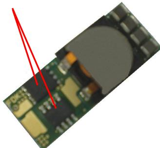
Fig. D: Location of the thermocouples for thermal testing
