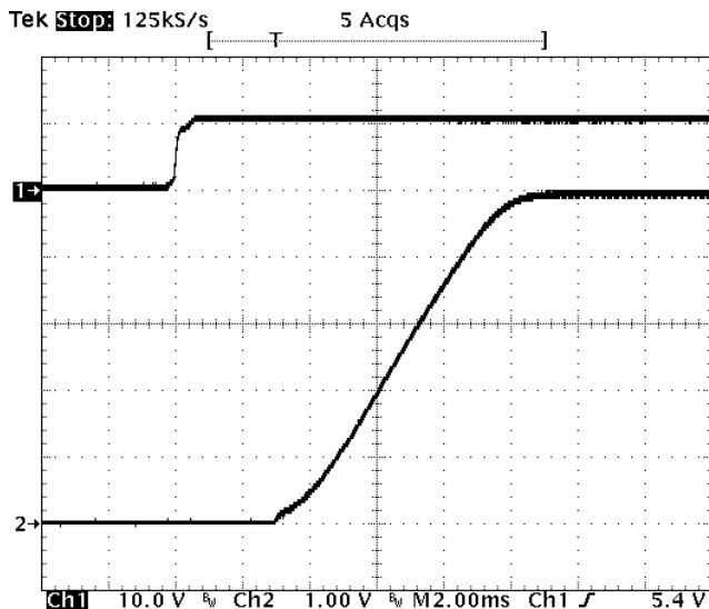
**Fig-5.0V-4:** Turn-on transient for  $V_{out}=5.0V$  with application of  $V_{in}$  at full rated load current (resistive) and  $47\mu Fx2$  external capacitance at  $V_{in}=12V$ .
