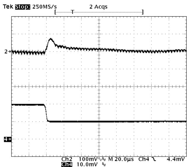
**Fig-1.0V-7:** Output voltage response for  $V_{out}=1.0V$  to negative load current step change from 10A to 5A with slew rate of  $-5A/\mu s$  at  $V_{in}=12V$ .  $C_o=47\mu Fx2$  ceramic.
