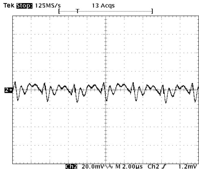
**Fig-1.0V-5:** Output voltage ripple (20mV/div.) for  $V_{out}=1.0V$  at full rated load current into a resistive load with external capacitance  $47\mu Fx2$  ceramic +  $1\mu F$  ceramic at  $V_{in}=12V$ .
