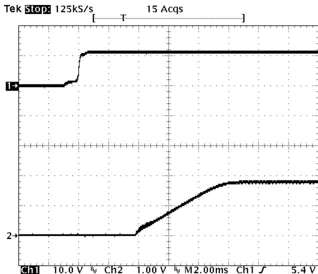
**Fig-1.8V-4:** Turn-on transient for  $V_{out}=1.8V$  with application of  $V_{in}$  at full rated load current (resistive) and  $47\mu Fx2$  external capacitance at  $V_{in}=12V$ .
