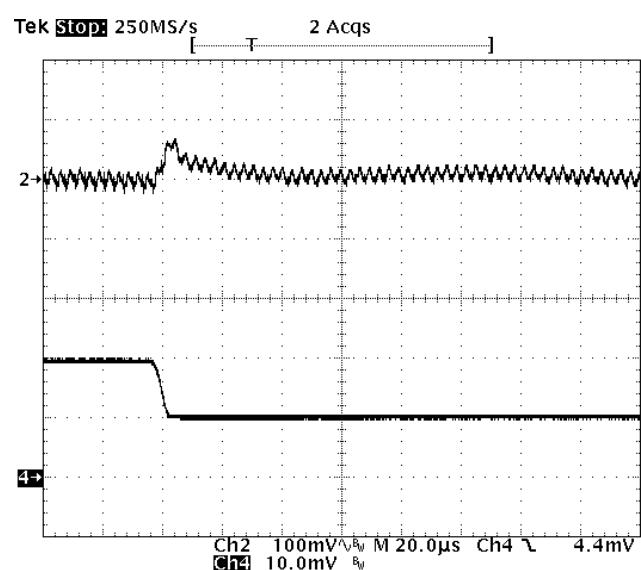
**Fig-3.3V-7:** Output voltage response for  $V_{out}=3.3V$  to negative load current step change from 10A to 5A with slew rate of  $-5A/\mu s$  at  $V_{in}=12V$ .  $C_o=47\mu Fx2$  ceramic.
