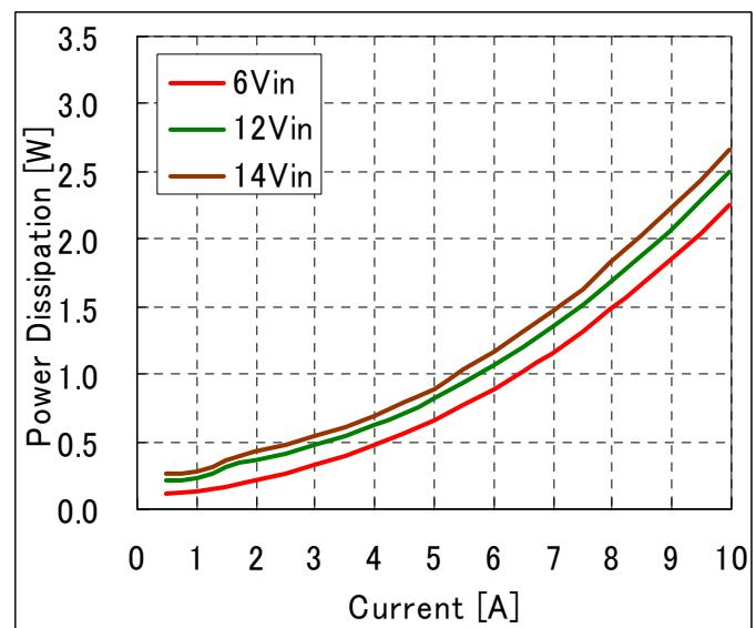
**Fig-1.0V-3:** Power Loss vs. load current and input voltage for  $V_{out}=1.0V$ .
