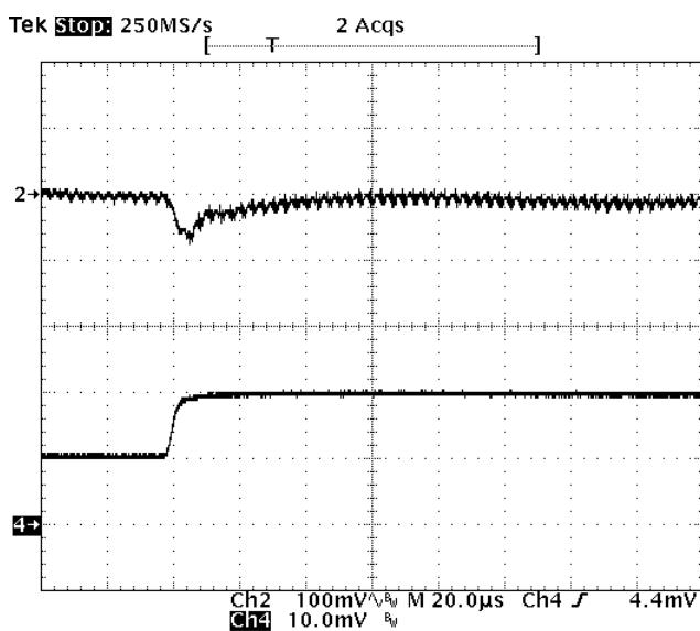
**Fig-1.0V-6:** Output voltage response for  $V_{out}=1.0V$  to positive load current step change from 5A to 10A with slew rate of  $5A/\mu s$  at  $V_{in}=12V$ .  $C_o=47\mu Fx2$  ceramic.
