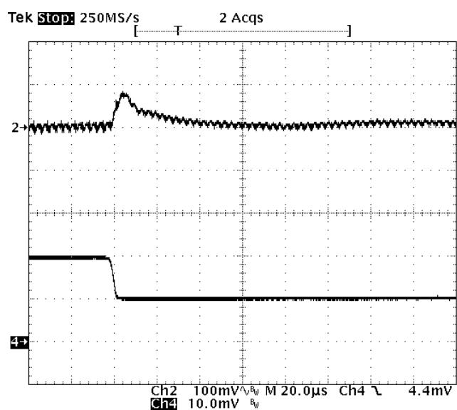
**Fig-1.2V-7:** Output voltage response for  $V_{out}=1.2V$  to negative load current step change from  $10A$  to  $5A$  with slew rate of  $-5A/\mu s$  at  $V_{in}=12V$ .  $C_o=47\mu Fx2$  ceramic.
