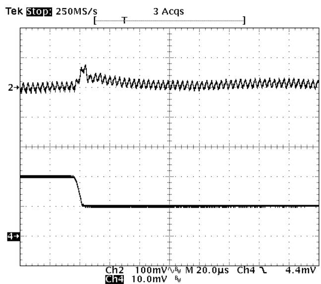
**Fig-5.0V-7:** Output voltage response for  $V_{out}=5.0V$  to negative load current step change from 10A to 5A with slew rate of  $-5A/\mu s$  at  $V_{in}=12V$ .  $C_o=47\mu Fx2$  ceramic.
