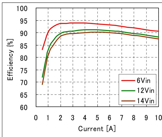
**Fig-2.0V-2:** Efficiency vs. load current and input voltage for  $V_{out}=2.0V$ .
