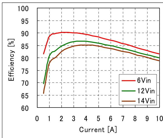
**Fig-1.0V-2:** Efficiency vs. load current and input voltage for  $V_{out}=1.0V$ .
