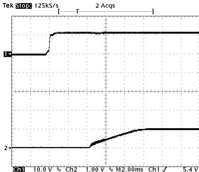
**Fig-1.0V-4:** Turn-on transient for  $V_{out}=1.0V$  with application of  $V_{in}$  at full rated load current (resistive) and  $47\mu Fx2$  external capacitance at  $V_{in}=12V$ .
